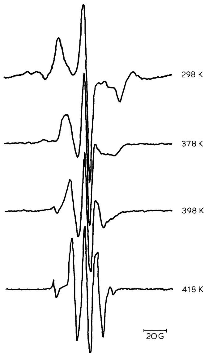
Figure 2 E.s.r. spectra of spin trapped polyethylene subjected to \gamma -irradiation. Temperatures of observations are indicated at right hand sides of respective spectra
